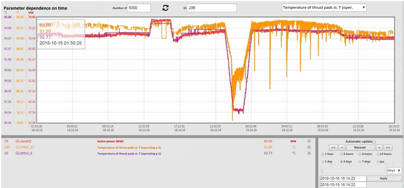
Fig. 1 Temperature of GT-1 thrust pads (oper. p.1 and p.2)
